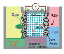
Peroxide power: Neutral solutions of H<sub>2</sub>O<sub>2</sub> can be produced directly and safely from O2 and H2 by using a fuel cell reaction. The most active and efficient cathode is a vapour-grown carbon fibre (VGCF) electrode coated with Co-tetraphenylporphyrin (0.05 wt%) on VGCF (2 mg cm<sup>-2</sup>). A maximum concentration of 13.5 wt% (4.0 M)  $H_2O_2$  is obtained under optimized conditions at 278 K.
